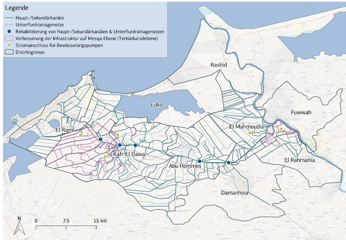
Figure 1 Illustration of project measures in the Mahmoudia irrigation area; source: own illustration based on georeferenced data supplied by the implementing agency.
