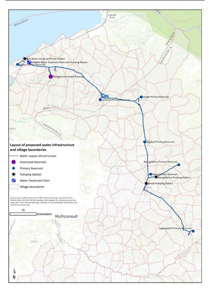
Figure 2: Routing of water main for Phase 1 with new locations of water treatment plant and reservoirs.
